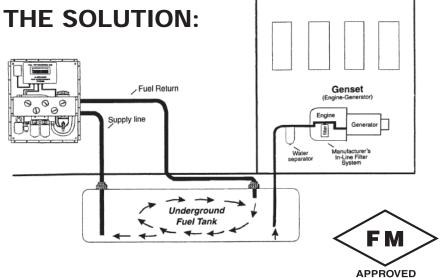
Install an FTI Automated Diesel Fuel Maintenance System to maintain clean quality and function in your fuel. Since you can't predict an emergency, the only way to be prepared is to prevent problems.
