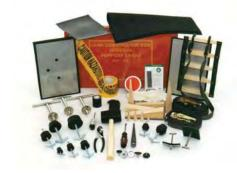
**Kit AE:** Contains items for larger holes, cracks and gashes in addition to the standard items listed above. These include one 8" x 12" stainless steel plate lined with 3/4" thick soft neoprene material and three T-bolts with preassembled wingnut washer combos. A second 8" x 12" stainless steel neoprene backed plate is included with hardwood cribbing ladder patch and two 22' heavy-duty nylon straps.
