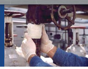
The STOP IT® Pipe Repair System includes a strong knitted fiberglass tape coated with fast setting urethane resins that are water activated. The system also includes FIX STIX™, a steel filled hand moldable epoxy that sets rock hard in only 20 minutes.
