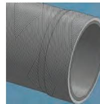
**Bondstrand 5000** is available in 1"-16" diameters with temperature range up to 200°F (93°C). This is a custom vinyl ester pipe available in Asia, Europe and South America and is recommended for most chlorinated and acidic mixtures. This pipe is manufactured with a 50 mil liner.
