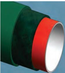
**Fiberspar LinePipe** products are continuous spoolable piping systems with HDPE liners over wrapped with a glass fiber epoxy thermoset matrix for corrosive and abrasive applications up to 2500 psi and up to 180°F. Diameters are available in 2 1/2" through 6 1/2" and continuous lengths up to 2 miles. A down hole version is also available.
