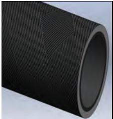
**Silver Streak** products are made for tough abrasive applications such as Flue Gas Desulfurization. This product is available from 1" through 48" diameters with a pressure rating up to 225 psig and a temperature rating up to 225°F (107°C).
