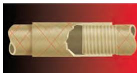
**T.A.B.™** - Threaded and bonded joining system. Double-lead threads provide quick and secure adhesive connections. Available for 2" through 6" **Red Thread** pipe sizes.
