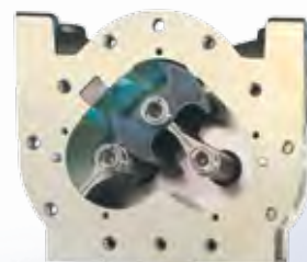
LC's three-rotor positive displacement measuring chamber.
