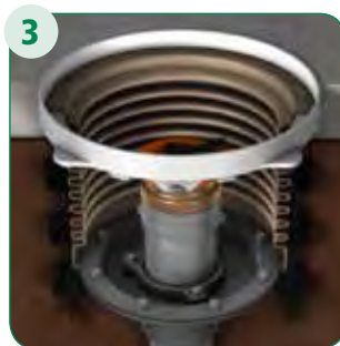
Replace Bellows, Reinstall Upper and Lower Rings
