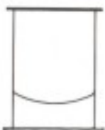
Model C-OVDS Open Vertical Dished Skirted
