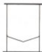
Model C-OVCS Open Vertical, Cone Skirted
