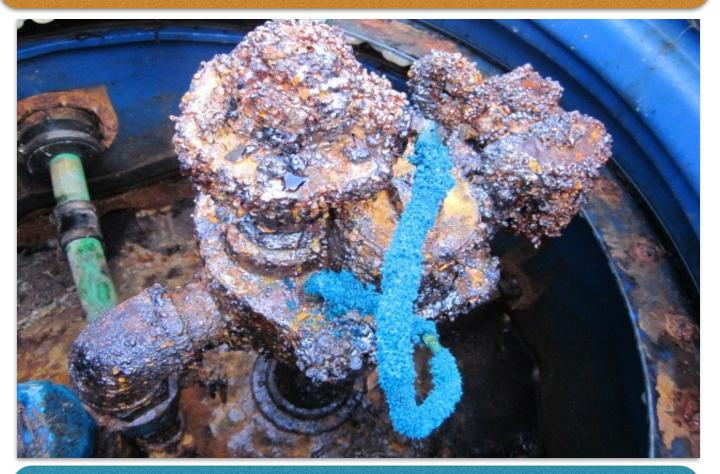
Bacteria, Water and Acetic Acid are Corroding your STP Sumps.
