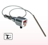
Switching Range: -58...250°F t<sub>max</sub> 250°F; p<sub>max</sub> 1,150 PSIG Connection: 6 mm dia. Smooth Probe 2 Transistor Switches
