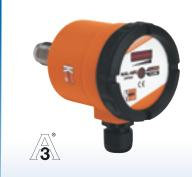
Water: 0.15...6.6 ft/sec t<sub>max</sub> 175 °F; p<sub>max</sub> 1,450 PSIG Connection: 1/2"...3/4" NPT, 1-1/2" Tri-Clamp® Linearity: ±10% of Full Scale
