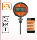
Measuring Ranges: -200...850 °C p<sub>max</sub> 34 bar Display: 6-Digit LCD Fittings: 1/4"...1/2" NPT, G 1/4...G 1/2, Compression Fitting Accuracy: ± 0.1% of Reading + 0.2°C
