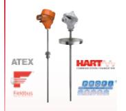
Measuring Range: -200...1,100 °C p<sub>max</sub> 3,625 PSIG Sensor: Pt100, 4-20 mA Connection: 1/2"...1" NPT, G 1/2...1, DIN 15 - 50 Flanges Output: Analog 4-20 mA
