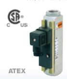
Water: 0.075...0.25 GPM to 1...14 GPM Air: 0.2...1.1 SCFM to 3...70 SCFM t<sub>max</sub> 240 °F; p<sub>max</sub> 5,000 PSIG Connection: 1/4"...3/4" NPT Accuracy: ± 5% of Full Scale
