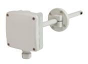
Air: 0...2,000/3,000/4,000 ft/min Output Signal: 0-10  $V_{DC}$  or 4-20 mA Supply Voltage: 24  $V_{AC/DC}$  Connection: Mounting Adapter Accuracy:  $\pm$  (0.2 m/s + 3% of Reading)
