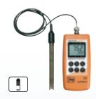
pH Measuring Range: 0...14 Measuring Range: 0...200 µS/cm to 0...200 mS/cm
