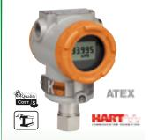
Measuring Range: -14.5...21.7 to 0...8,700 PSIG Power Supply: 12-45 V<sub>DC</sub> Connection: 1/2" NPT Accuracy: ± 0.075% of Full Scale
