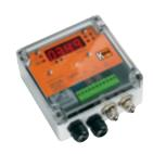
Measuring Range: 0...20" H,0 Power Supply: 24 V<sub>AC/DC</sub>, 110 V<sub>AC</sub>, 230 V<sub>AC</sub> Display: 4-Digit LED Connection: 1/4" NPT or 6x8 mm Tube Accuracy: ±1.0% of Full Scale
