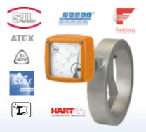
Water: 6.6...26.4 GPM to 880...6,600 GPM t<sub>max</sub> 570 °F; p<sub>max</sub> 580 PSIG Connection: 1-1/2"...20" ANSI Wafer Accuracy: ± 2.5% of Full Scale
