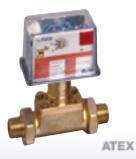
Water: 0.8...14.5 GPM to 13.2...158 GPM t<sub>max</sub> 210 °F; p<sub>max</sub> 230 PSIG Connection: 1/2"...2" NPT, 1/2"...2" ANSI Accuracy: ± 3 - 5% of Full Scale
