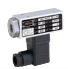
Switching Range: -14.5...0 PSIG to 580...6,100 PSIG Overpressure: 1.4 - 5 Times Connection: 1/4" NPT Repeatability: ± 3 - 4% of Full Scale
