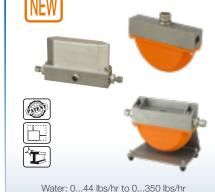
Water: 0...44 lbs/hr to 0...350 lbs/hr t<sub>max</sub> 350 °F; p<sub>max</sub> 5,800/8,700 PSIG Connection: 1/2" NPT, Gryolock/Swagelok Accuracy: ±0.15% of Reading
