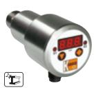
Measuring Range: -30"...0" Hg to 0...5,800 PSIG Display: 3-Digit LED Power Supply: 24 V<sub>DC</sub> Connection: 1/4" NPT. 1/2" NPT Accuracy: ± 0.5% - 1.0% of Full Scale
