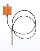
Measuring Range: 0...100% rH; 0...200°C t<sub>max</sub> 200°C; p<sub>max</sub> 25 bar Outputs: 2x 4-20 mA Accuracy: ±2% rH
