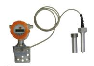
Water: 3.3...33 ft/sec t<sub>max</sub>100 °C; p<sub>max</sub> PN 16 Connection: ANSI 3"...16", Weld-on Nozzle ø 40 mm, Sensor with Union Nut M52x2 for Pipelines DN 80...400 Accuracy: ± 1.5% of Full Scale
