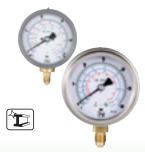
Measuring Range: -1...9 to -1...40 bar Housing Ø: 63, 100, 160 mm Overload Protection: 1.0 Times Connection: 7/16-20 UNF, G 1/4 Accuracy: ±1.0% or ±1.6% of Full Scale
