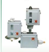
Switching Range: -14.5...0 PSIG to 135...435 PSIG Overpressure: 1.5 - 5 Times Repeatability: ± 0.25% of Full Scale
