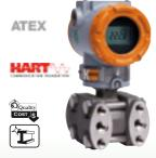
Measuring Range: 0.3"...6" WC to 60...6,000 PSIG Power Supply: 18-45 V<sub>DC</sub> Connection: 1/4" NPT, 1/2" NPT Accuracy: ± 0.075% of Full Scale
