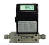
Air: 0...10 SCCM to 0...500 SLPM t<sub>max</sub> 120 °F; p<sub>max</sub> 500 PSIG Connection: 1/4" NPT, 1/2" NPT; 1/4" or 1/2" Swagelok<sup>®</sup> Accuracy: ±1.5% of Full Scale
