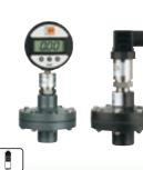
DSD...DRM-630 and SEN...DRM-631 Meas. Range: 0...20 to 0...145 PSIG Housing Ø: 74 mm Connection: 1/2" NPT Accuracy: ±1.0% of Full Scale
