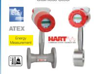
Water: 0.89...22 GPM to 141...4,270 GPM Air: 1.8...18 SCFM to 2,071...203,000 SCFM t<sub>range</sub> -328...750 °F; p<sub>max</sub> 1,450 PSIG Connection: 1/2"...8" ANSI Option: Integrated Temperature and Pressure Sensor, Wafer Type Accuracy: ±1% Reading for Gas & Steam, ± 0.7% Reading for Liquids
