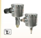
Dielectric Constant<sub>min</sub>: 20 t<sub>max</sub> 212 °F; p<sub>max</sub> 145 PSIG Connection: G 1/2, Tri-Clamp® Open-Collector
