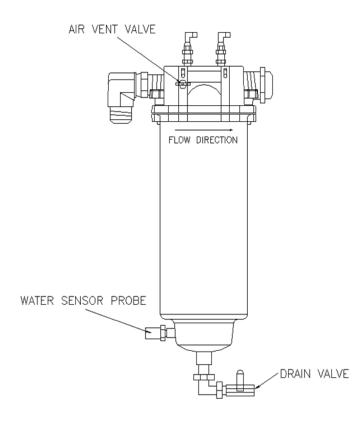
If, after draining the water separator, the alarm continues while restarting system, unplug water level sensor cable located near the bottom of filter housing. Restart system and run for several minutes to clean metal elements of the water sensor. Plug cable in and check system.
