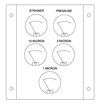
Each switch gauge monitors the filter identified in the above diagram and offers an ongoing visual status of system pressure, vacuum and each of the filters condition.
