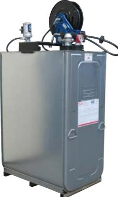
DWT110M    | DWT110P                                                                             | Double Wall Tank, Graco Dispense Pkg (3:1 LD Pump, SD Reel with 50' Hose, Meter, Air Pressure Regulator), Down Tube, Fluid Level Gauge, Lockable Fill Cap with Vent, Pump/Reel Bracket                       | 110 Gallons | 28"W x 29"D x 68"H |
